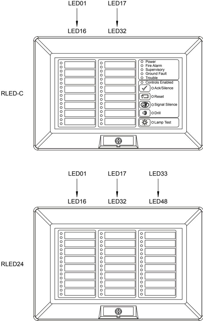
Figure 10: GCI card LED and switch numbering
