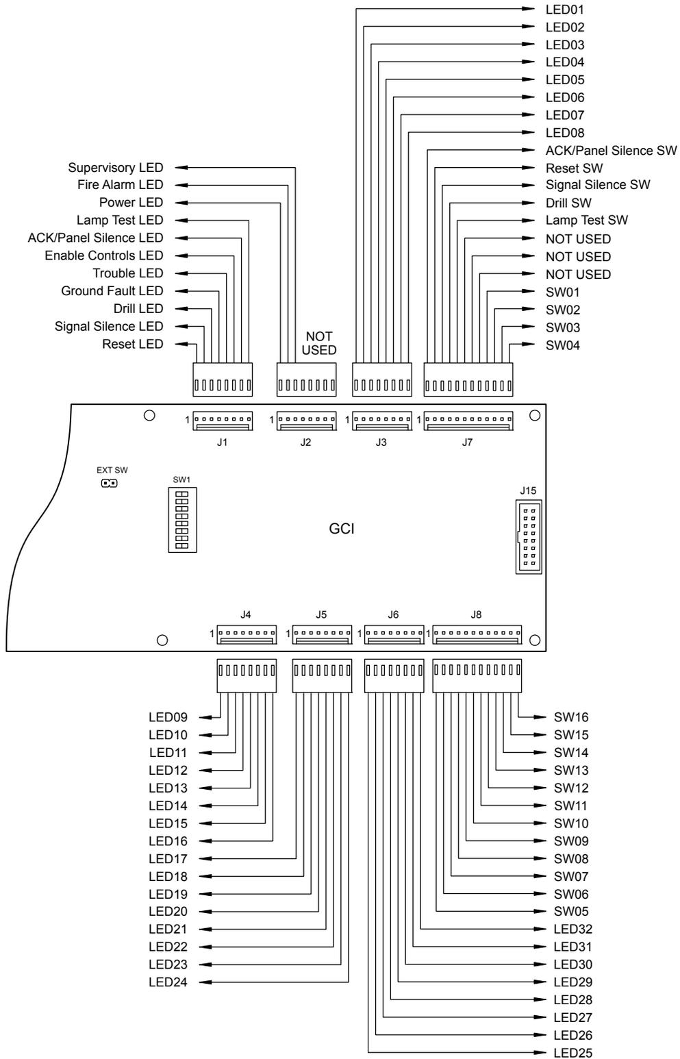
Figure 11: GCIX card LED and switch numbering
